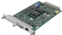
MANAGEMENT CARD MANAGEMENT VIA THE CONSOLE PORT, OR ETHERNET PORT USING SNMP OR TELNET
